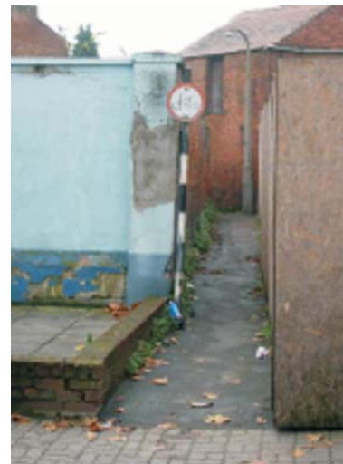
This unattractive footpath link has limited opportunities for natural surveillance, is too narrow, and has an awkward turn at the top. As such it provides opportunities for crime and anti social behaviour.
