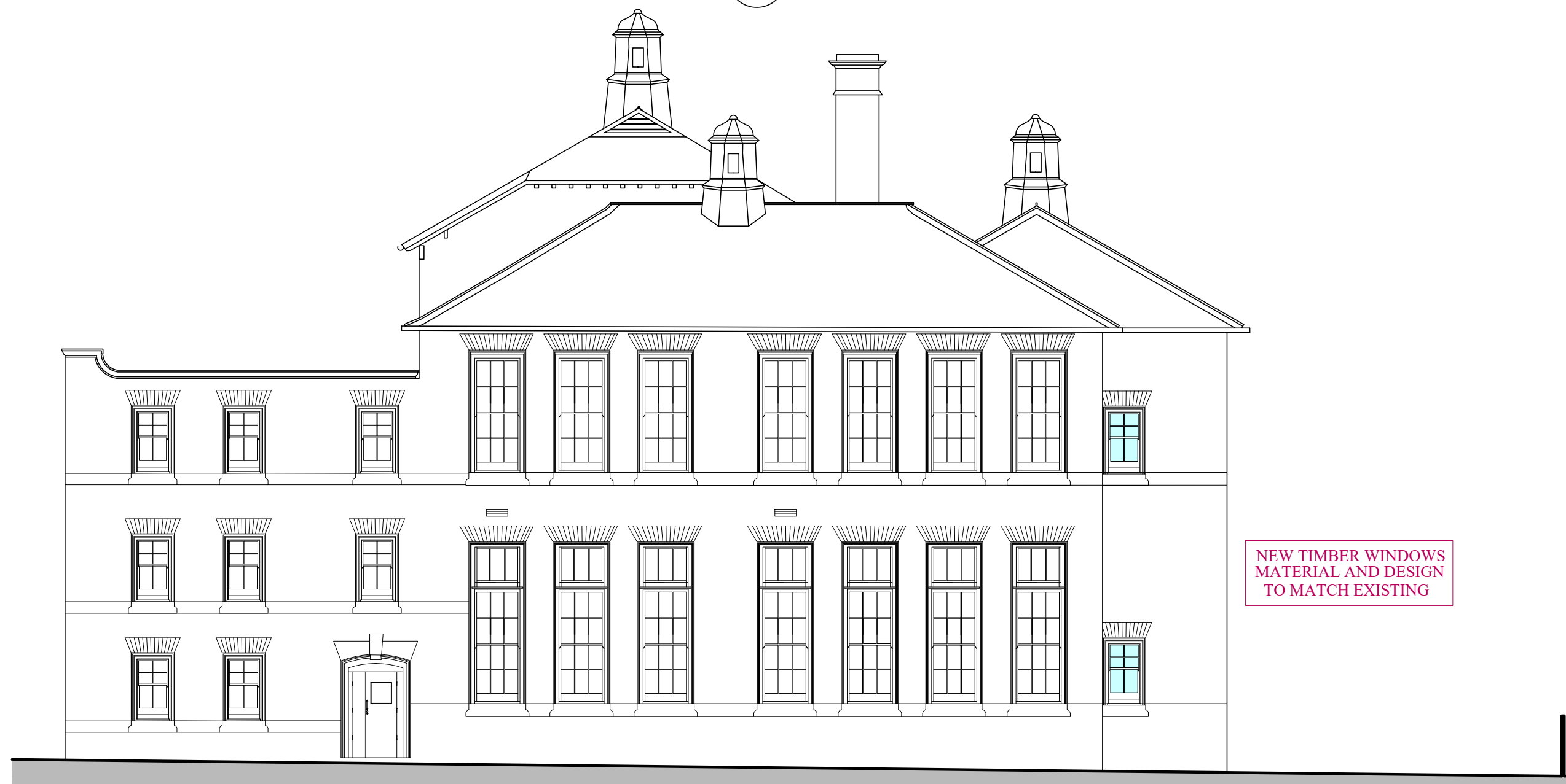
- EAST ELEVATION - SCALE 1:100
