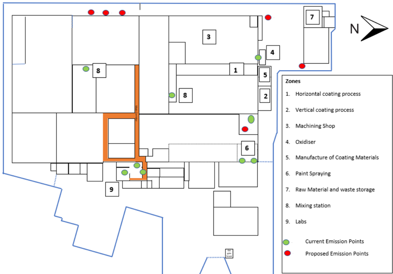
Figure 3.2 Permali Process Locations and Emission Points
