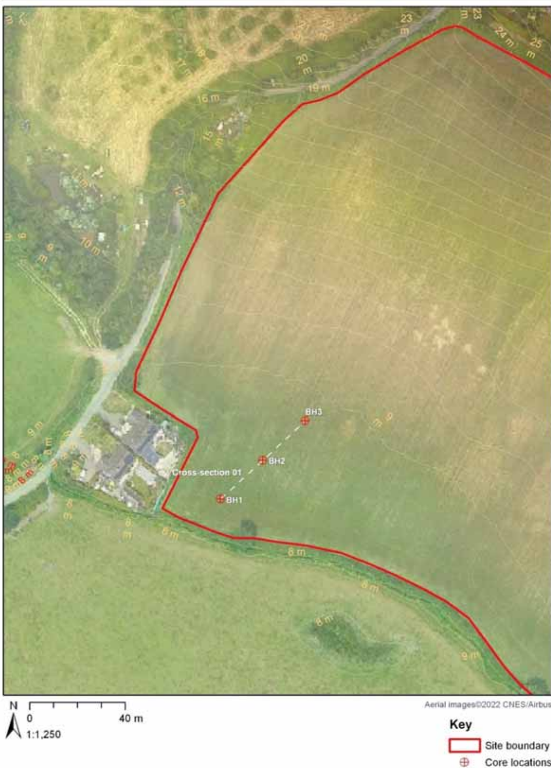
Fig. 01: Site plan showing the south west corner of the Site and the location of the three geoarchaeological boreholes and LiDAR derived topography (© Environment Agency copyright and database right 2015. All rights reserved.)
