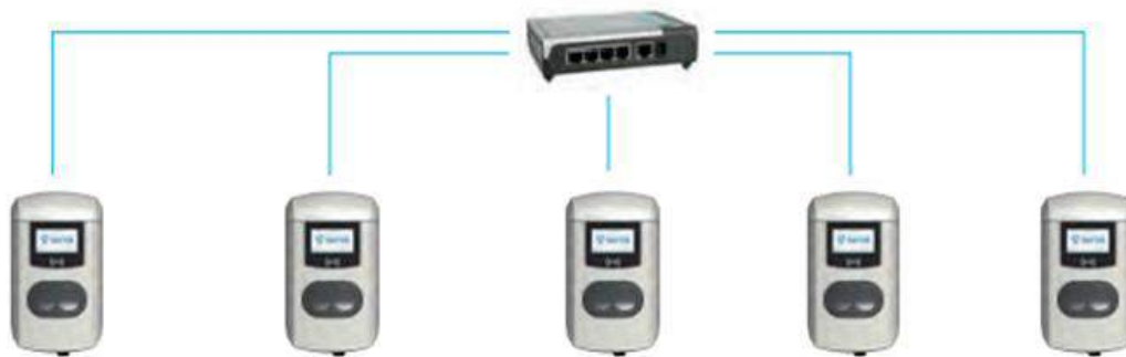
TYPICAL NETWORKED CAT 6 SMART CHARGING
