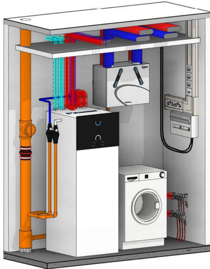
TYPICAL UTILITY CUPBOARD WITH ELECTRICAL CONSUMER UNIT
