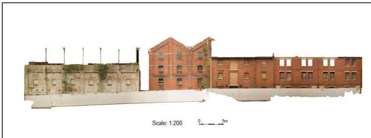
Fig.2 Photogrammetric rendition of the east elevation of the complex, with High Orchard Street Silo on the far left (reproduced from the 2018 Final Report, where it is provided at scale)
