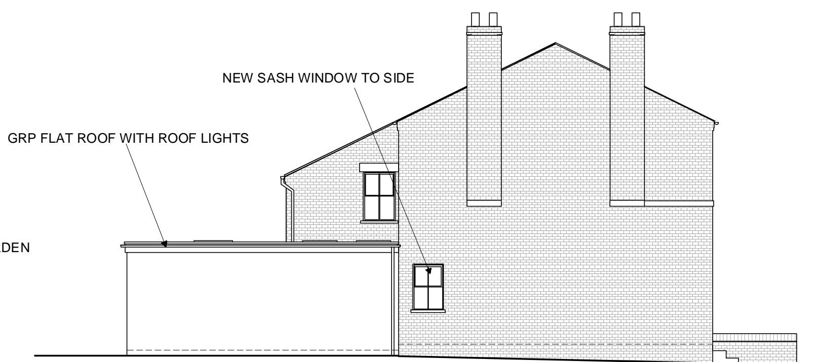
AS PROPOSED SIDE ELEVATION - 1:100
