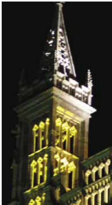
Existing floodlights (right) to be replaced by narrow-beam projectors aimed at the triangular sections of the pinnacles; and the effect of a single projector seen above
