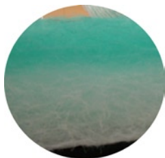
CROSS SECTION OF THE GLASS FIBRE MEDIA USED IN TYPE 90 PANEL FILTERS
