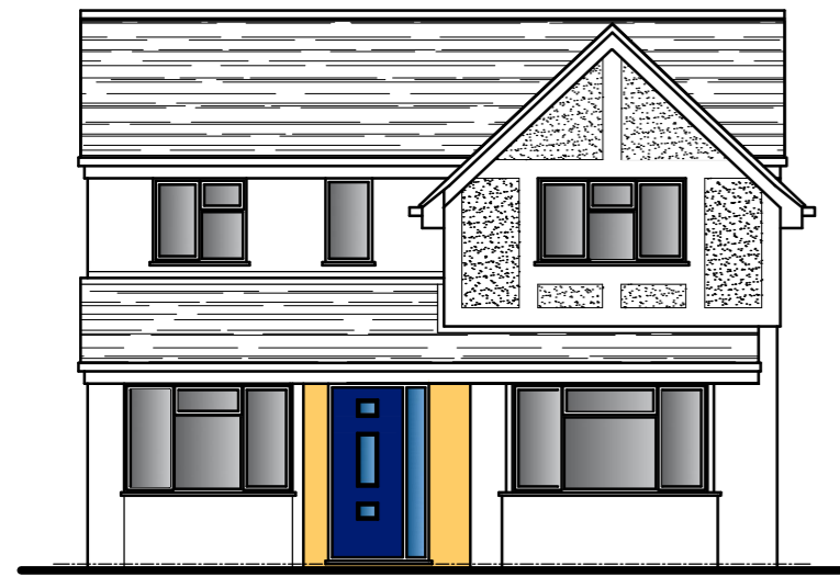
Proposed Front Elevation Existing doorway moved to new location fitted within new external wall construction to match the existing.
