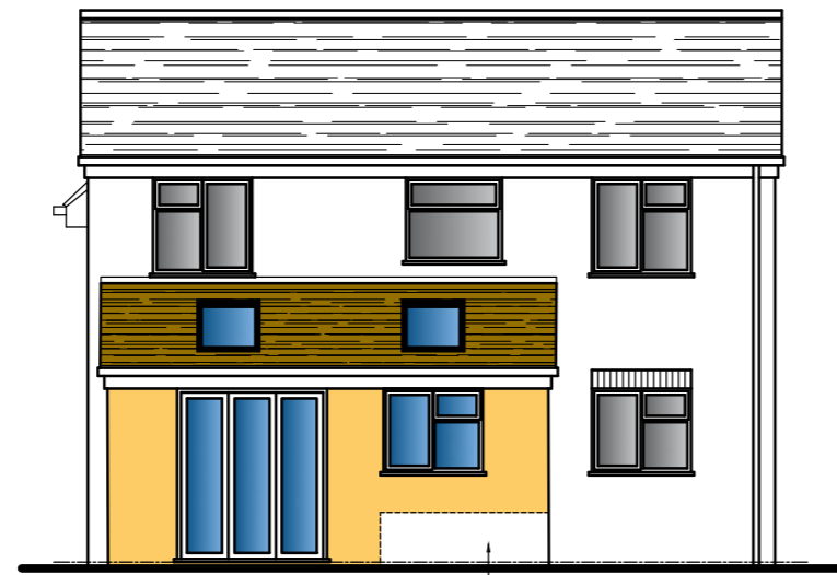
Proposed Rear Elevation Existing partial wall construction to remain from original Conservatory.
