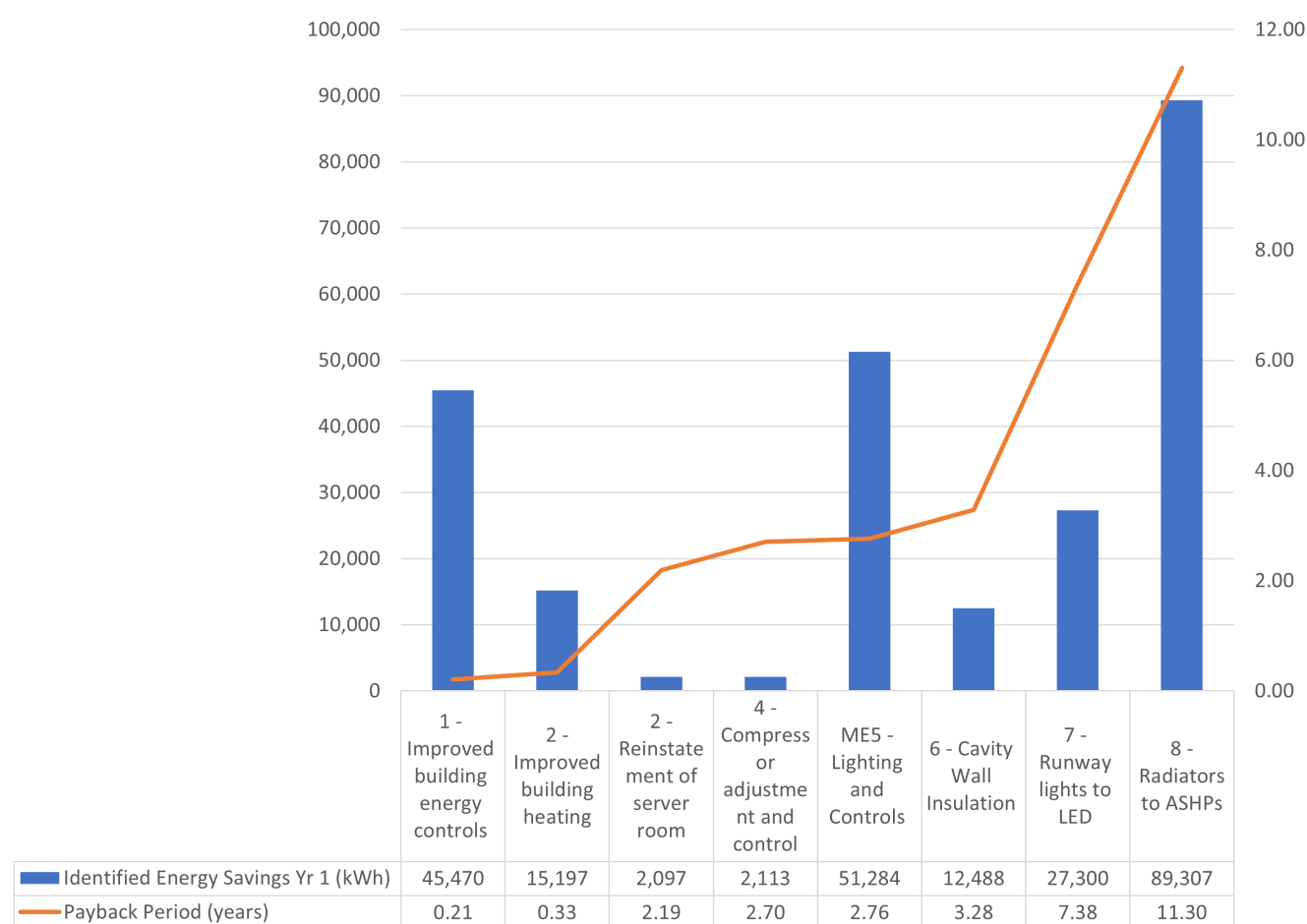
Figure 4-16. Energy savings and payback period - energy efficiency actions for Gloucestershire Airport Estate. Source: CLS Energy Ltd adapted by WSP.
