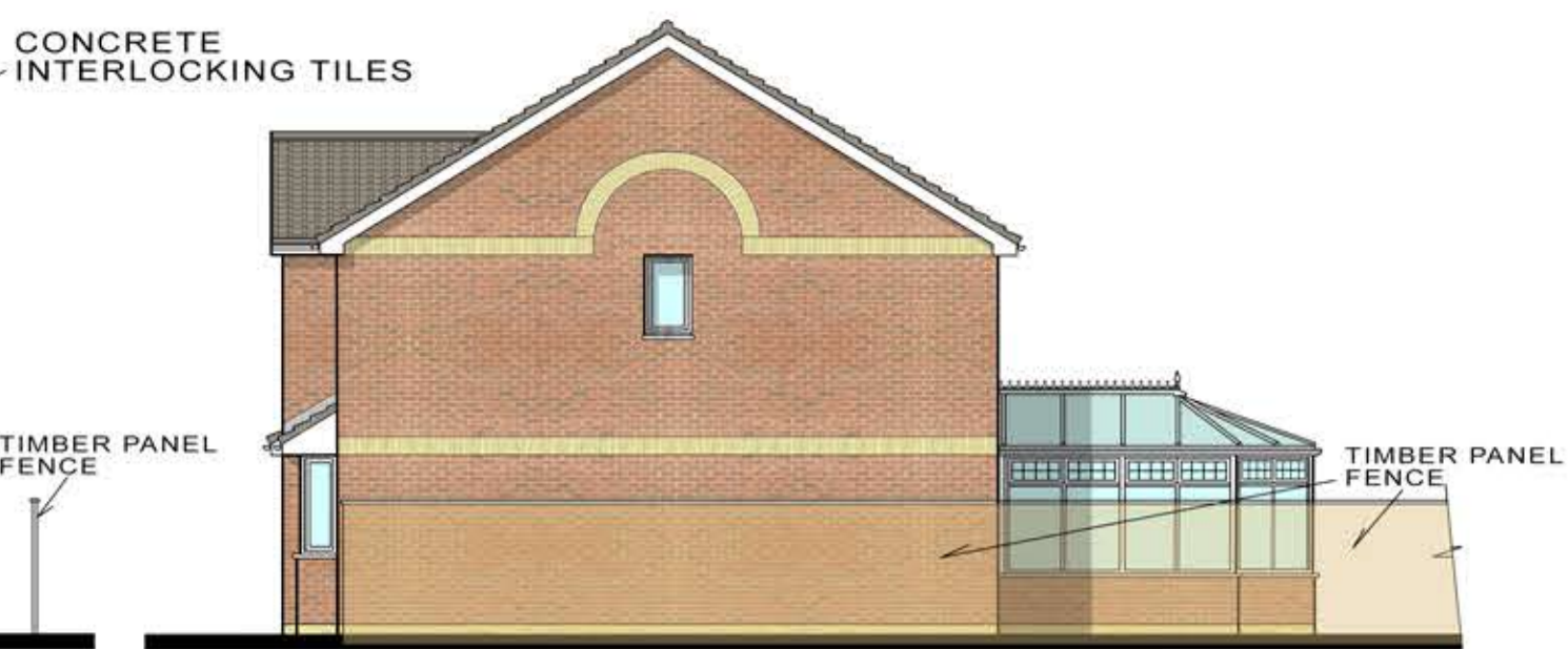
EXISTING SIDE ELEVATION WEST 1:100
