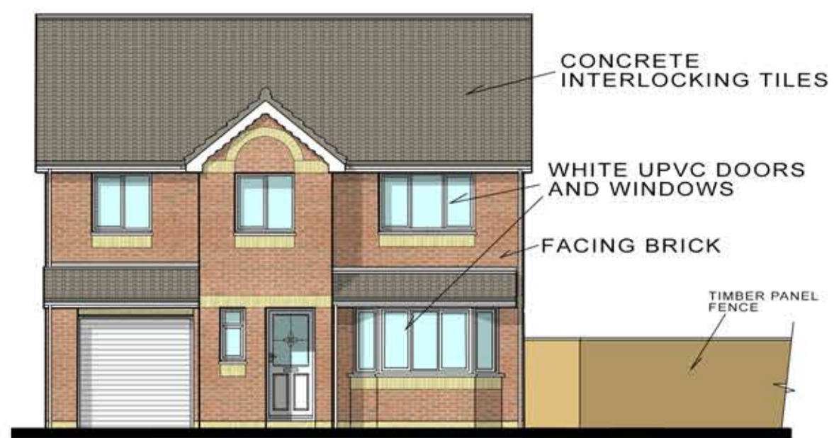
EXISTING FRONT ELEVATION NORTH 1:100
