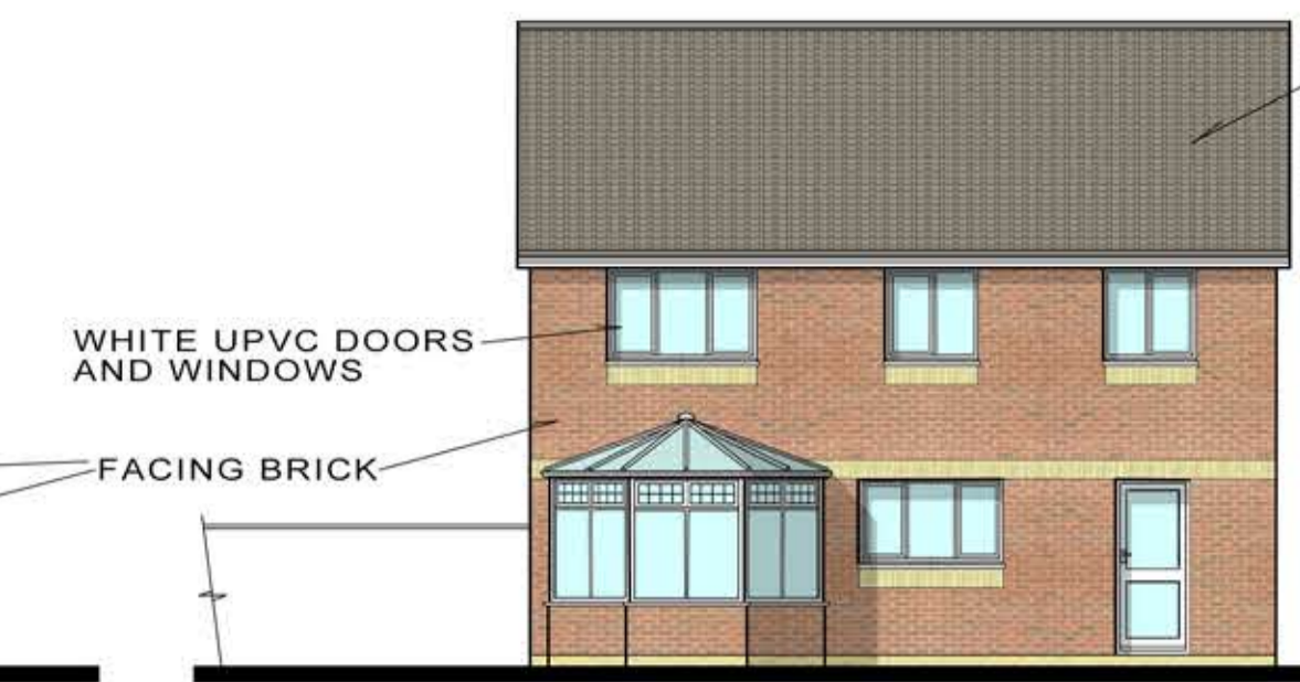
EXISTING REAR ELEVATION SOUTH 1:100
