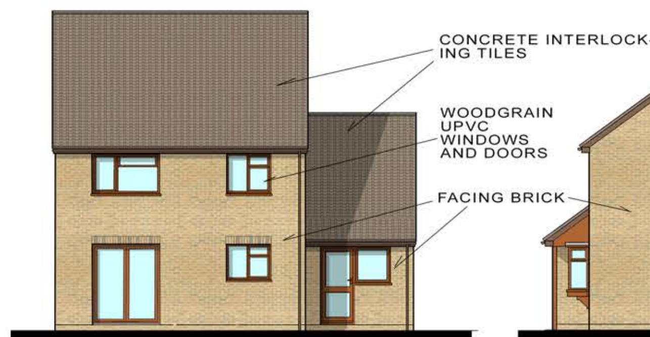
EXISTING REAR ELEVATION NORTHWEST 1:100
