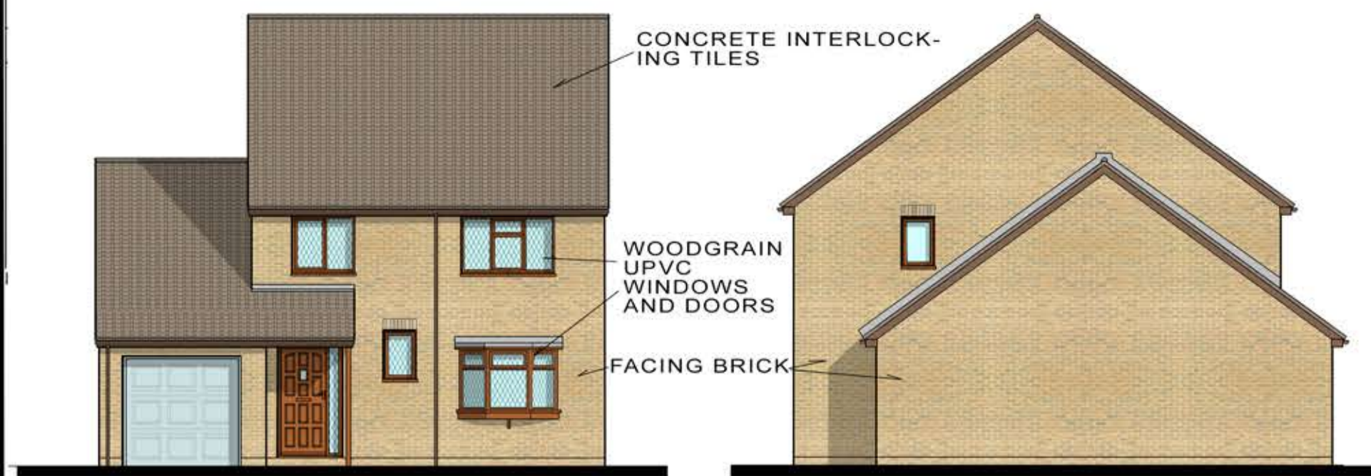
EXISTING FRONT ELEVATION SOUTHEAST 1:100
