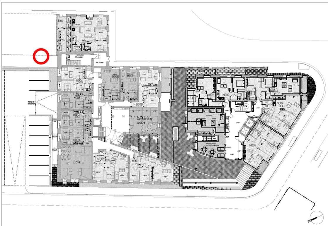
Mark-Up Showing Location of 2no. Small Air Conditioning Units at 4.5 m & 6.5 m Above Ground Level
