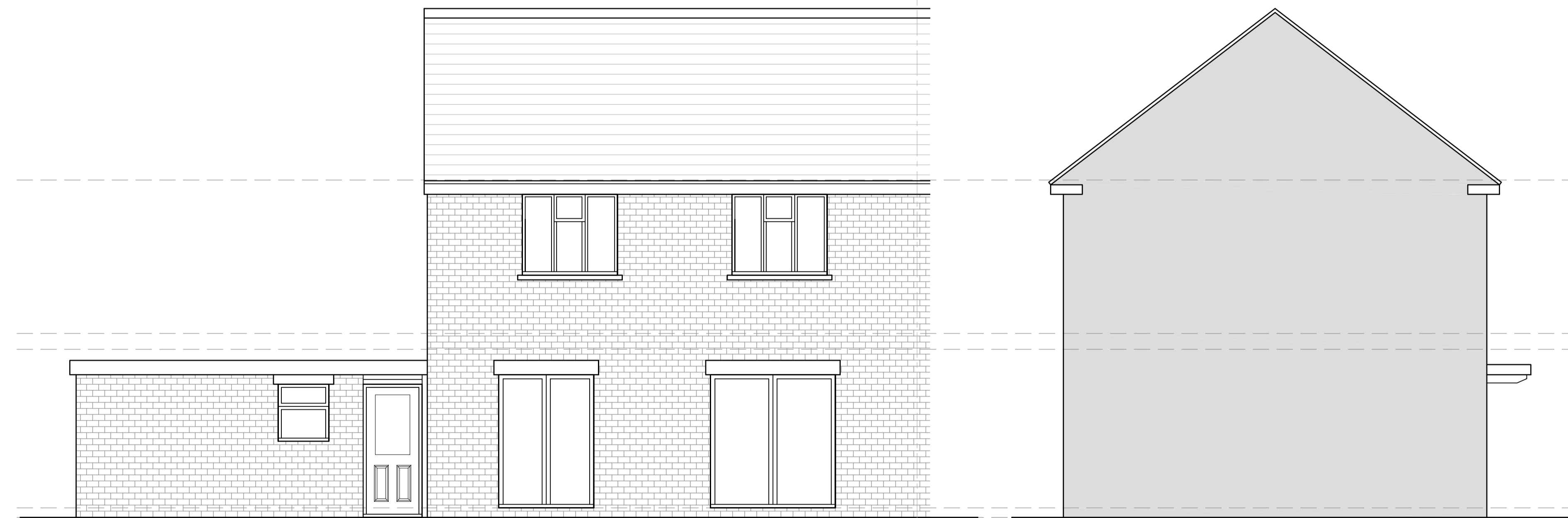
EXISTING REAR ELEVATION
