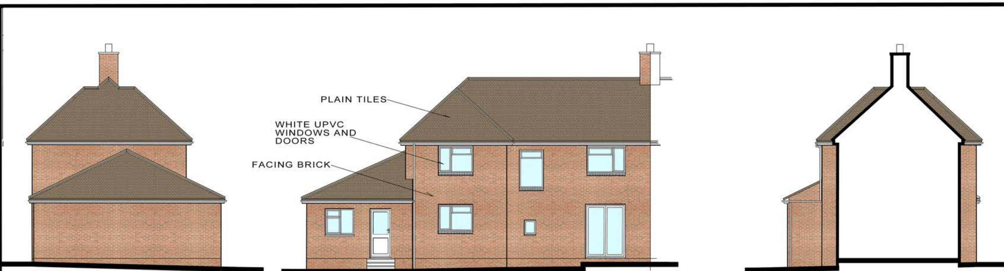
EXISTING SIDE ELEVATION NORTHWEST 1:100
