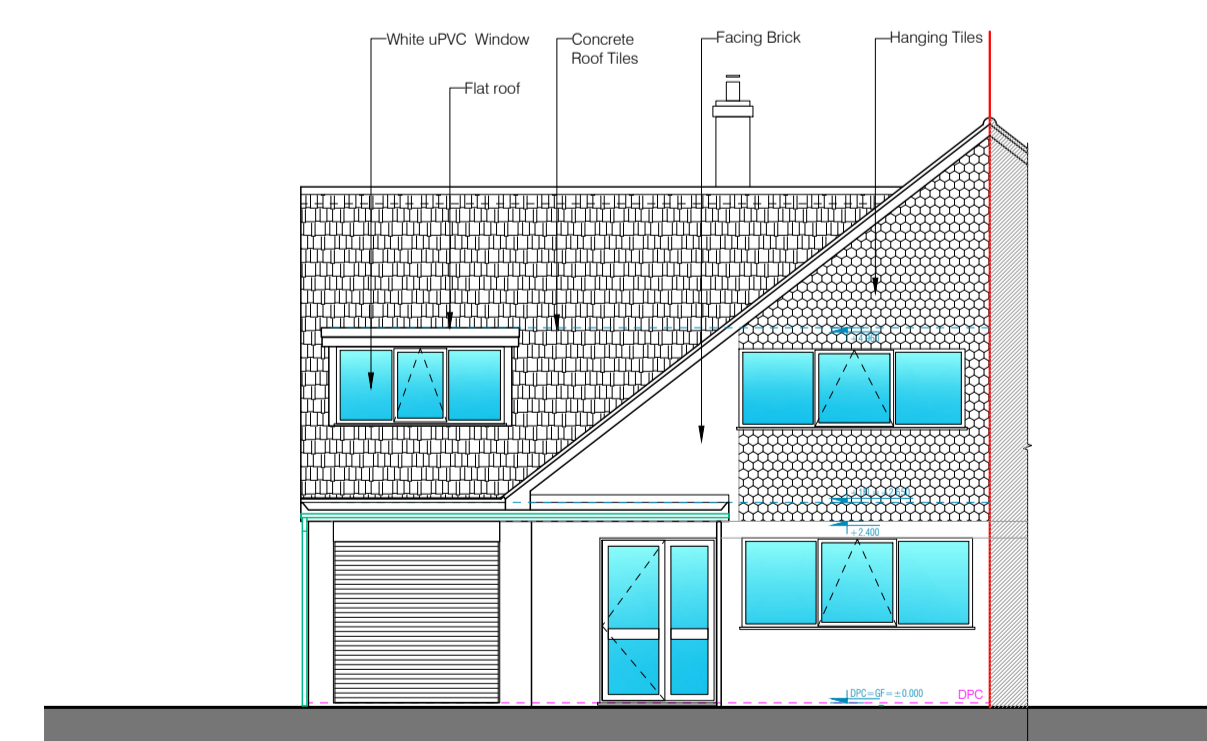
FRONT ELEVATION AS EXISTING SCALE - 1:100@A1
