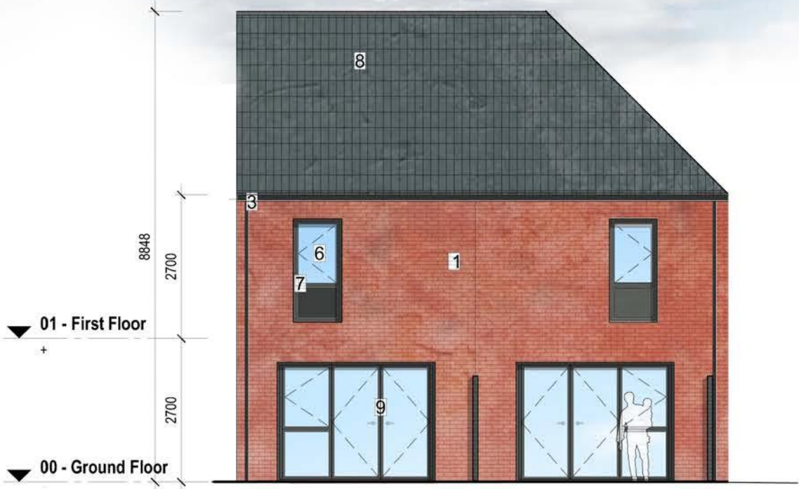
3 Townhouse 2B 3P Type 3 - Rear Elevation SCALE 1:50
