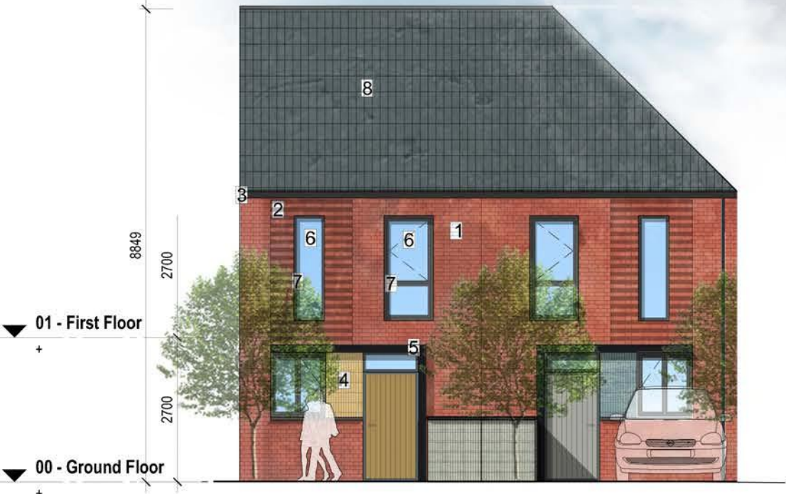
1 Townhouse 2B 3P Type 3 - Front Elevation SCALE 1:50
