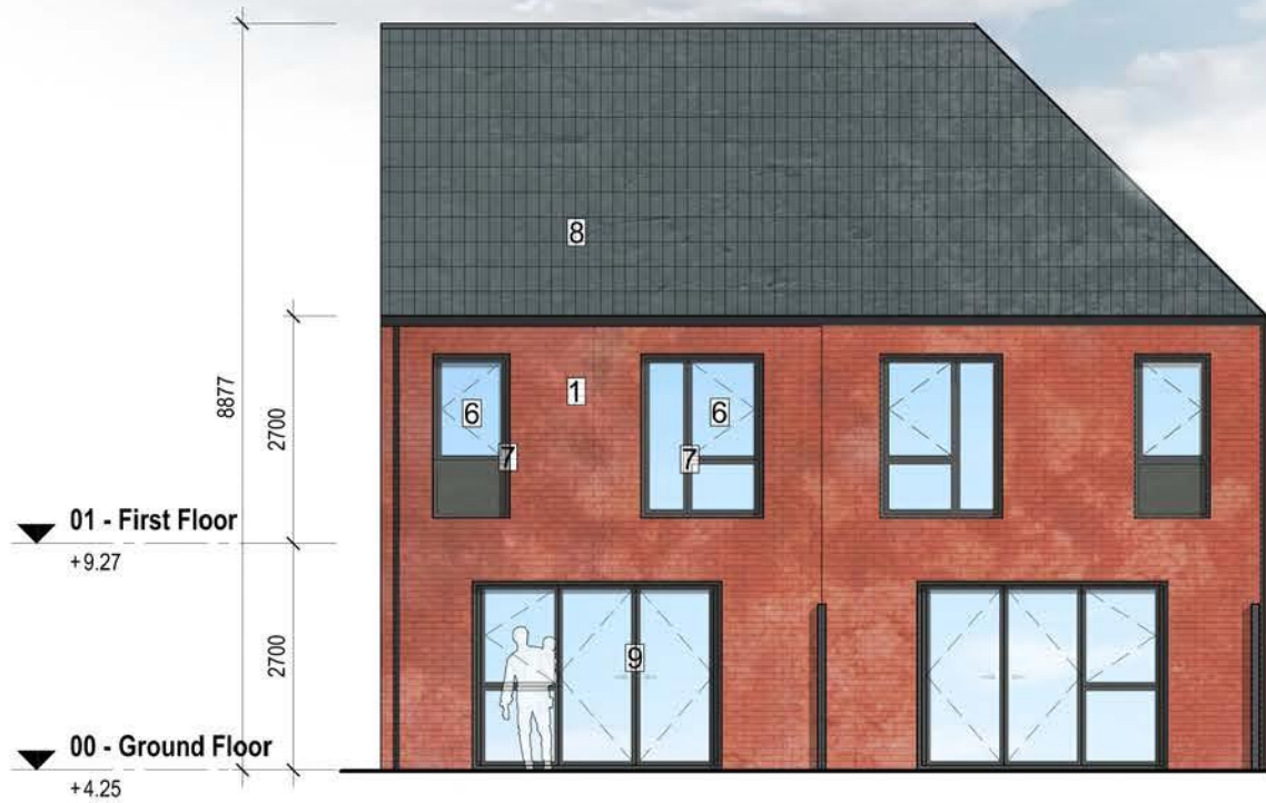
3 Townhouse 3B 5P Type 4 - Rear Elevation SCALE 1:50
