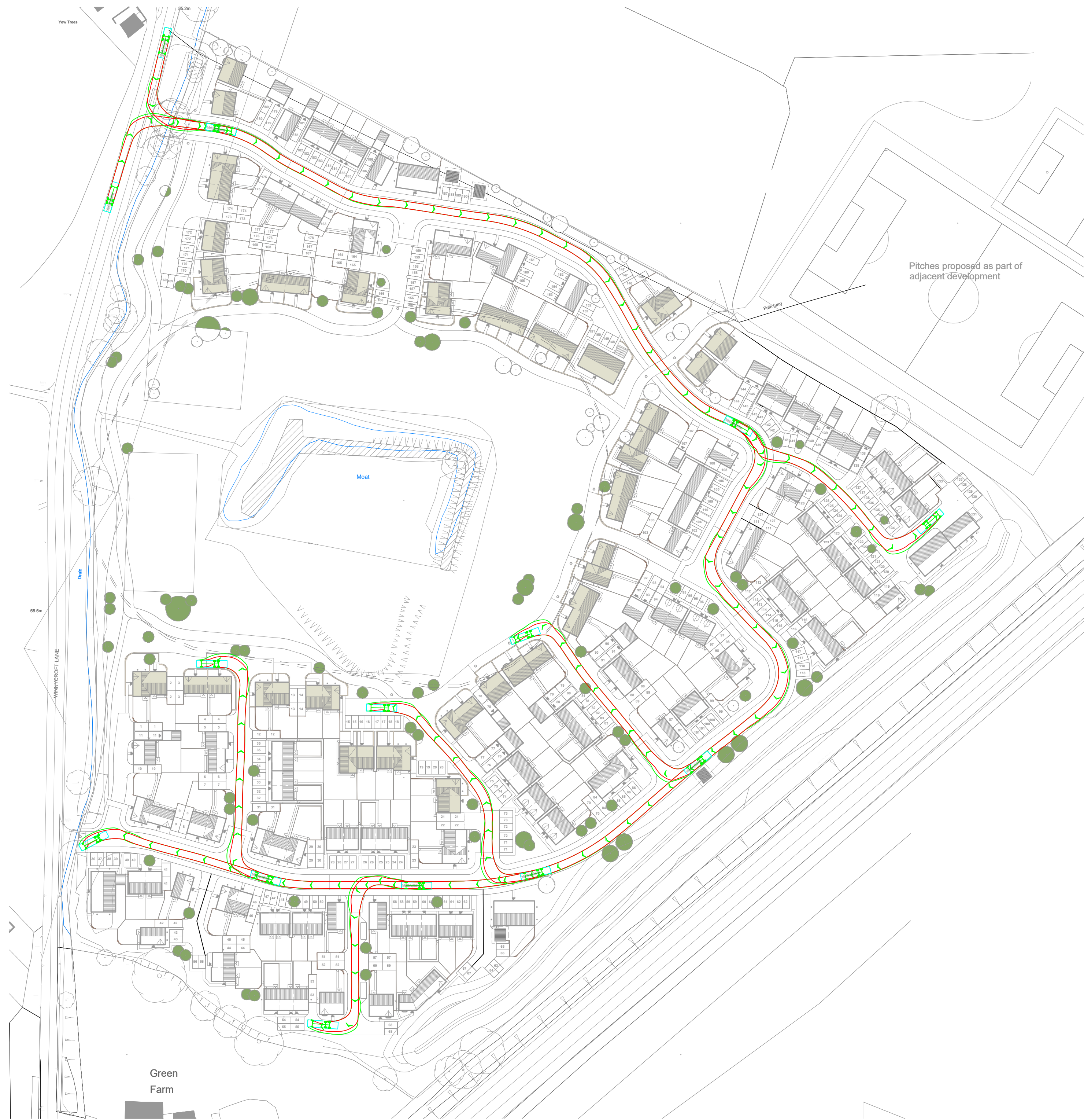
Swept Path Analysis of a 11m Refuse Vehicle Entering Site
