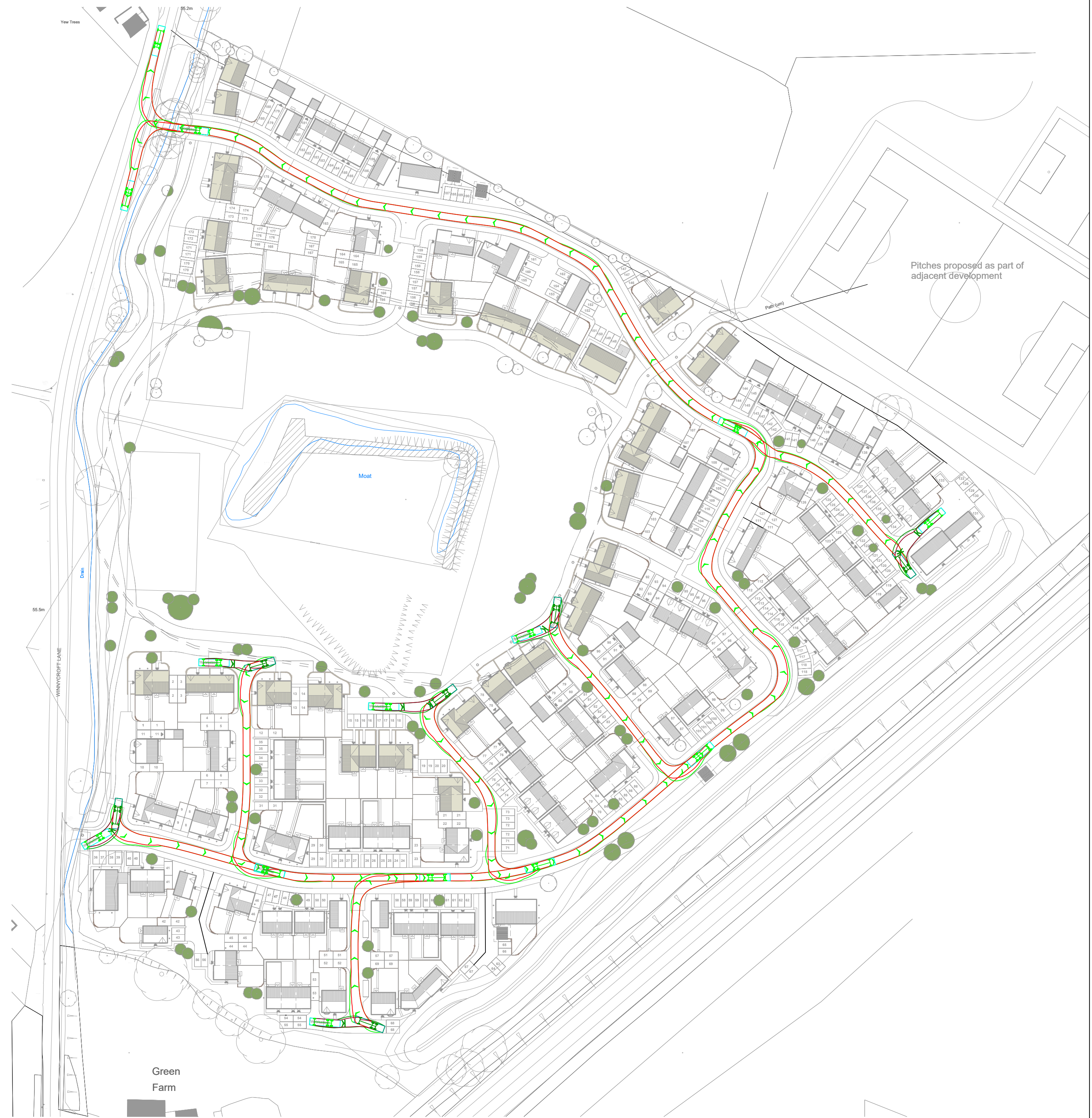
Swept Path Analysis of a 11m Refuse Vehicle Egressing Site
