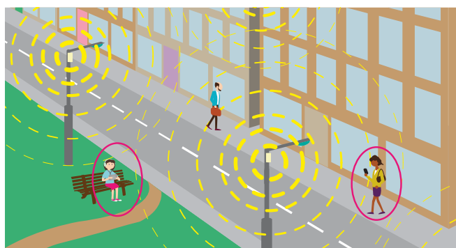
Figure B: Small cell deployment in a city centre
