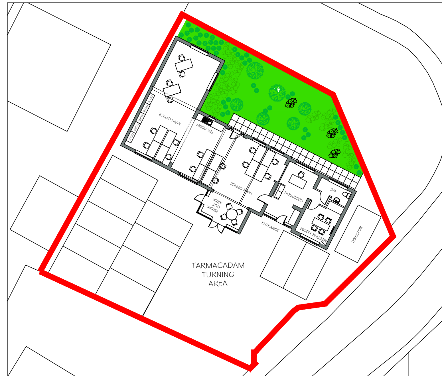
PROPOSED BLOCK PLAN. SCALE 1:200
