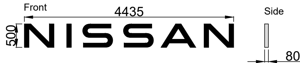
Sign C,D,P,Q: Nissan Wordmark Size 3 Individual 3D letters Face Illumination: Internally Illuminated with white LEDs Material: 1mm Hairline S/S Returns 4mm Black/White Acrylic Front Face Scale 1:50 @ A3
