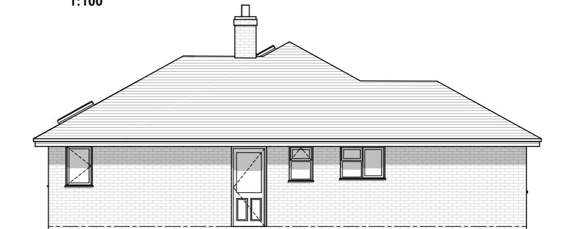
North West Elevation as Proposed 1:100
